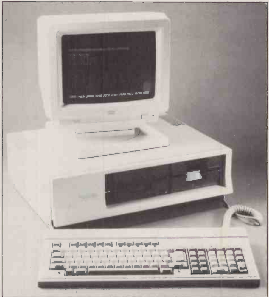
The 16S has a conventional three-box layout with a colour or monochrome monitor.
