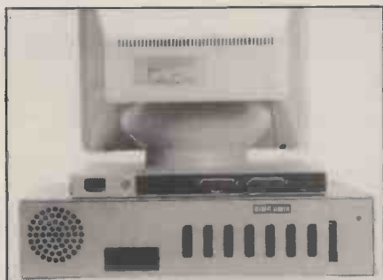
The Pinnacle supports up to seven terminals connected via the serial ports.
